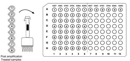
**Recommendation:** Use a new set of tips for each column. Alternatively use the same set of tips, but do not touch the bottom of the wells.
